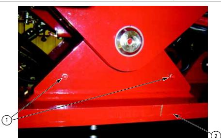
Figure 6-3: Fifth Wheel Bearing Grease Fittings
