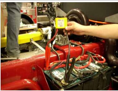
Figure 6-16: Connecting the Anti-Zap Device
