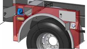
Figure 5-2: Typical DEF Reservoir Location
