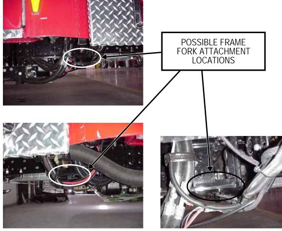
Figure 6-10: Possible Frame Fork Attachment Locations
