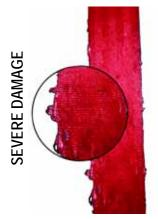
MAJOR / SEVERE DAMAGE, CUTS, RIPS, ABRASION, OR FRAYING
