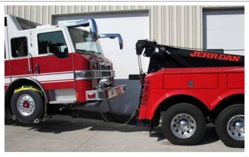
Figure 6-8: Underlift Device using Tire Lift Brackets
