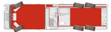
REAR OF VEHICLE SWINGS SLIGHTLY TO ACCOMPLISH OVERALL TIGHTER TURNING RADIUS
