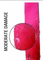
SIGNS OF CUTS, SIGNIFICANT ABRASION OR FRAYING
