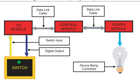
Figure 6-5: Pierce Multiplex System Operation
