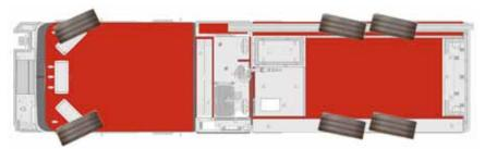
REAR OF VEHICLE SWINGS SLIGHTLY TO ACCOMPLISH OVERALL TIGHTER TURNING RADIUS
