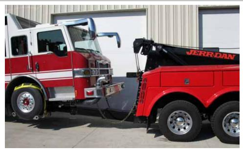
Figure 6-9: Underlift Device using Tire Lift Brackets
